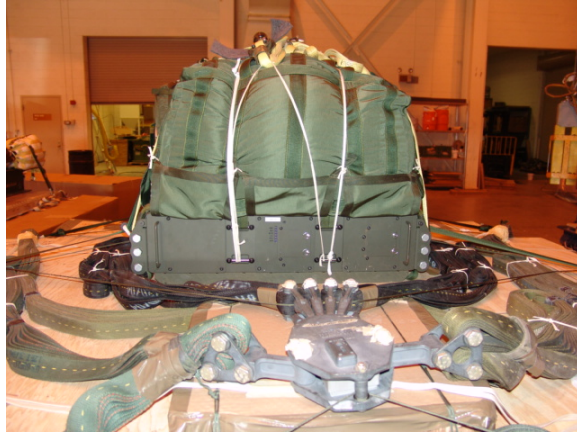
Figure 10: DRAGONFLY Deployment Bag and AGU Rigged to Load
