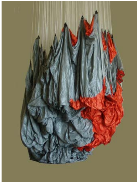
Figure 9: Main Canopy Hanging from Tower, Ready for Packing
