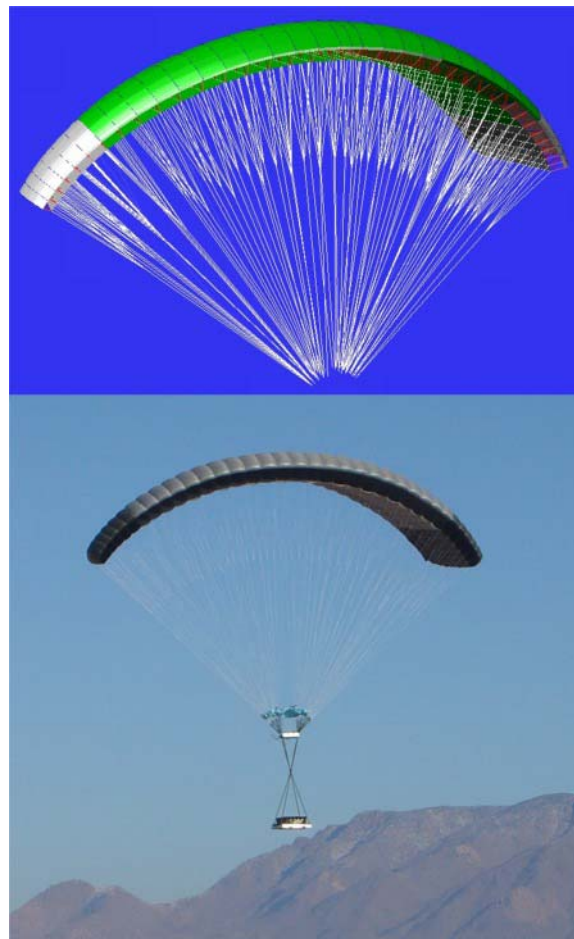
Figure 3: DRAGONFLY Main Canopy Model vs. In-Flight
