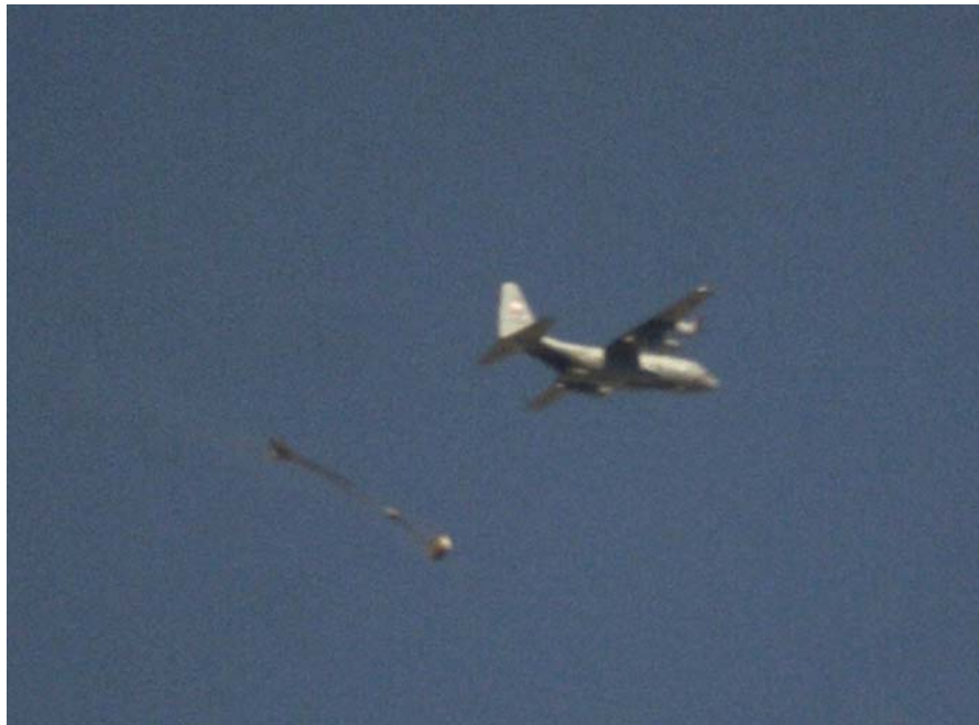
Figure 8: Reefed Drogue-fall, Sling Extension
