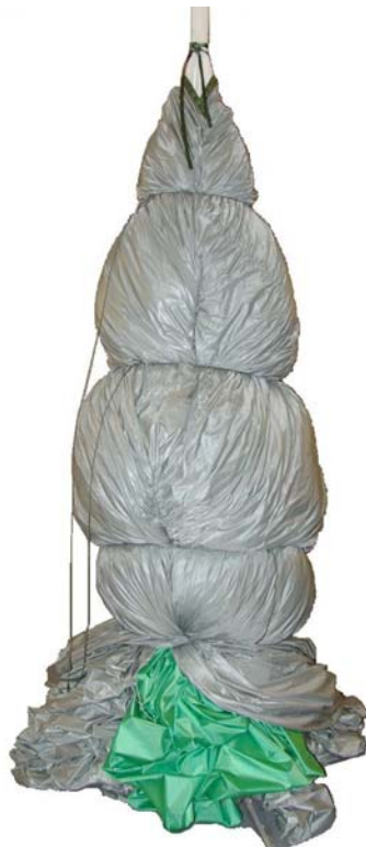
Figure 6: Main Canopy in Longfold, Ready for Folding into Deployment Bag
