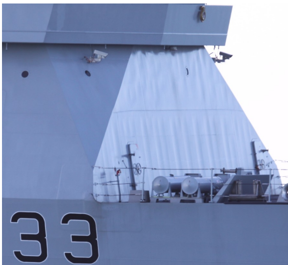
IDS300 launch tubes as fitted to UK RN Type 45 frigate
