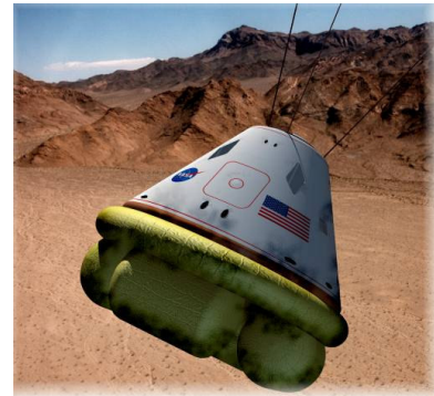
HANDOUT IMAGE SOFT LANDING: This rendering shows how the airbags would work on a capsule.
